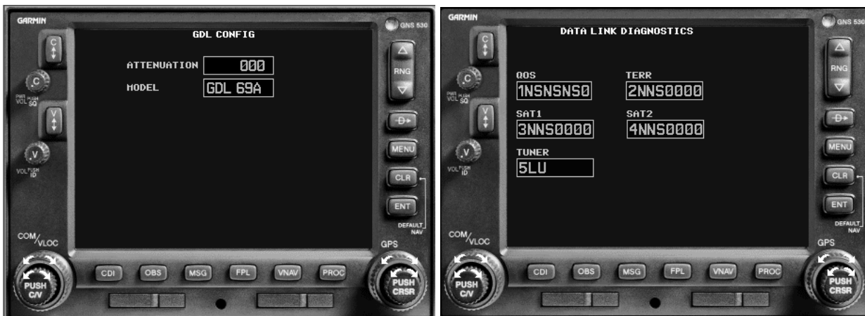
Figure 4-4. Data Link Configuration Page on the 400W/500W Series (500W Series shown, 400W Series screen is similar)
